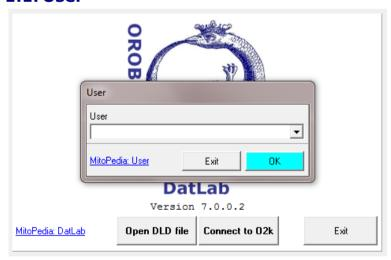
For better documentation and traceability, a user name has to be entered selected after or starting DatLab. The current user is displayed in the O2k signal line. User names are connected with personal layouts (see graph Layout menu).
