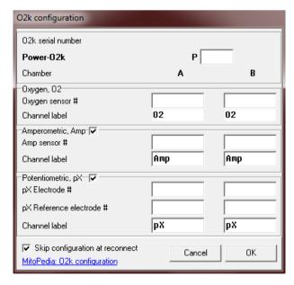
In  $\bigcirc$ xygraph-2k $\bigcirc$ O2k configuration, channels (Amperometric, Amp  $\boxtimes$ , Potentiometric, pX  $\boxtimes$ ) can be switched on/off by selecting the according tick box.
