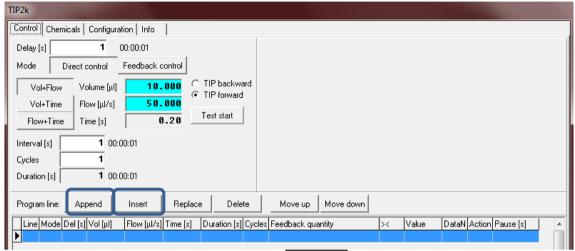
A new button Append improves user-friendly programming of the TIP2k, for adding a new line at the end of the programme. Insert adds a new line at the selected position.
