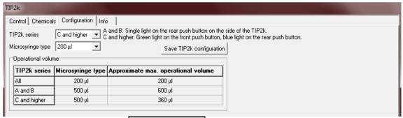
The tab <u>Configuration</u> accommodates the TIP2k series and Microsyringe type. Based on this information, DatLab checks the total volume programmed in the <u>Control</u> tab and warns the user if the approximate maximum operation volume is exceeded.
