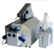
The OROBOROS Oxygraph-2k, with the Titration-Injection microPump (TIP2k) on top, and the Integrated Suction System (ISS) on the right.
