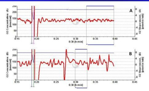
Equilibration is continued in the 'open chamber' at 27 °C and interrupted by a 'stirrer test' [F9]: the stirrers are switched off for 30 s, with automatic restart to 750 rpm. The signals of both sensors show a rapid response (blue traces). Equilibration chamber A is complete (at a slope of 0.7 pmol  $O_2 \cdot s^{-1} \cdot ml^{-1}$ ),
