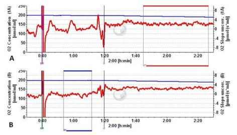
Stirrer test (40 min) and air calibration at 37 °C with phosphate buffer solution (mark, Graph B). The raw signals (Gain 1) were 2.27 V and 2.28 V (Table 3). Closing the chamber (C) and evaluation instrumental background oxygen flux at air saturation (mark J°1, Graph A): 2.16 and 2.38
