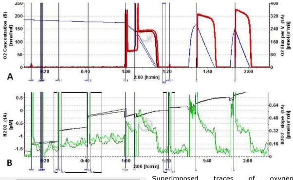
1.00-E 0.80-O.000 0.050 0.100 [µM] 0.150 0.200 Superimposed traces of oxygen concentration and respiration (Graph A) in phosphate buffer solution (PBS) and of  $H_2O_2$  equivalents and  $H_2O_2$  production (Graph B). During the first 1 h period, two steps were performed of  $H_2O_2$  calibration with two titrations of 0.1  $\mu$ M  $H_2O_2$  (Graph B, showing the step changes; Graph C linear regression). Graph layout 05; N=10 data points for slope calculation.. 2014-07-02 AB-02.DLD
