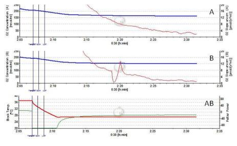
**Immediately** after preparation of new oxygen sensors (electrolyte and membrane application) the O2k was switched from 37 °C to 27°C (AB: red line). signal oxygen sensitive to temperature (blue lines; A and B for O2k-Chamber Α and В, respectively), thermal as well as
