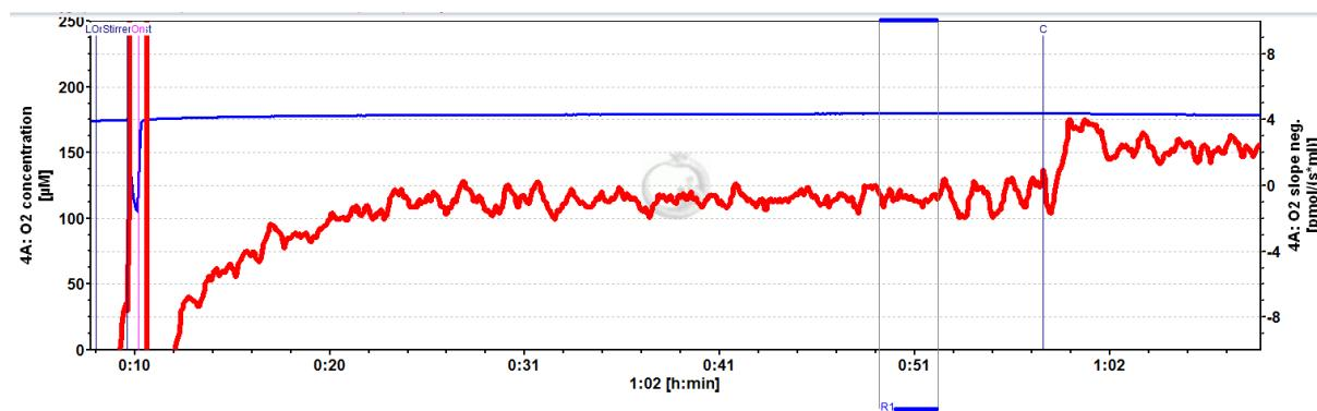
11. Calibrate at air saturation (R1) and copy calibration values to your calibration list for quality control (Excel file: [O2-calibration.xlsx](#)).
