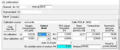
Or open <u>Calibration</u> and select an Oxygen channel. Or select an  $O_2$  Concentration plot and press [F5].
