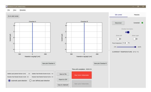
The cyclic voltammetry will automatically stop after finishing five cycles. Afterwards you have the option to Save to File (.dld8) and to Export to CSV (.csv). To copy the oxidation and reduction peak potential values, click on Copy to clipboard. The figures can be exported separately by clicking on Save plot Chamber A or B, and copied into a .doc or .ppt file.
