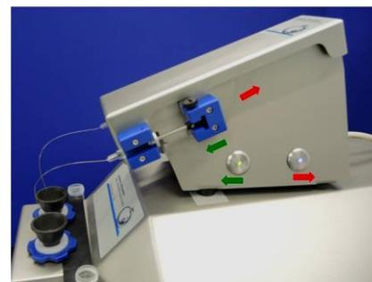
**Push buttons** are located on the right side of the TIP2k. Push the front one (green light) for forwards movement, and the rear one (blue light) for backwards movement of the plunger holder. For stopping the manual movement, simply release the push button. Pushing both buttons simultaneously also stops the pump. At manual operation of the TIP2k, the step motor moves at maximum speed.
